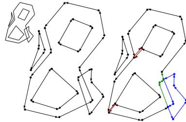
**Figure 3:** **Top Left:** Input shape defined as a set of connected vertices forming five outlines. **Middle:** Outlines converted to half edges. **Right:** The constraint outlines are merged with the respective outline (red half-edges), and the intersecting outlines are split editing the second large outline (green half-edges) and forming the third outline (blue half-edges)
