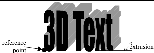
Figure 3-9 The Default Reference Point and Extrusion for a 3DText Object
